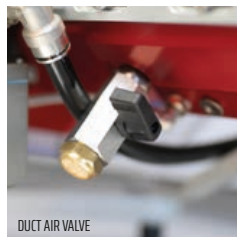
DUCT AIR VALVE
