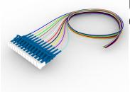
Fiber Optic Pigtail, 12 fibers, Singlemode, LC/UPC to Stub, 0.9 mm diameter, multicolor, 2m
