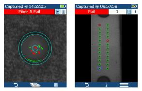
FOCIS Lightning focuses, captures and analyzes all fibers in the MPO/MPT end-face with a click of a button.
