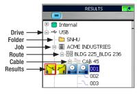
OTDR test results are saved in .SOR file format and displayed on the "file tree" as to con.
